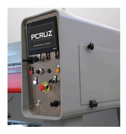
An interactive PC with a touch-screen and intuitive interface of **PCruz** proprietary **EasyEdge** software allows for easy handling of the machine. An operator can input full information on the jobs to be performed: type of the material, size, thikness, shape of the edge, as well as define the machining mode.
